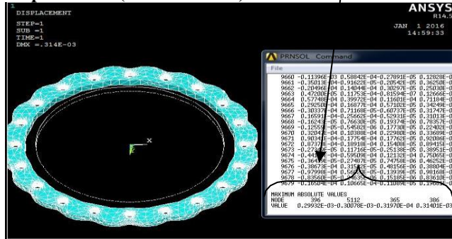
Fig 11: Displacement (nodal solution)
